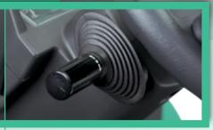
**Electric Shift Lever** Forward / neutral / reverse shift operation is easy with the touch of a finger.
