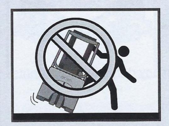
Do not try to jump off the truck in case of a tipover. Stay within the truck. Keep your seatbelt fastened, grip the steering wheel tightly, brace your feet, and lean away from the direction of fall.
