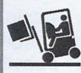
Tilting mast forward when forks are raised and loaded can tip the truck over causing injury or death. Do not tilt elevated load forward unless it is over a stack.
