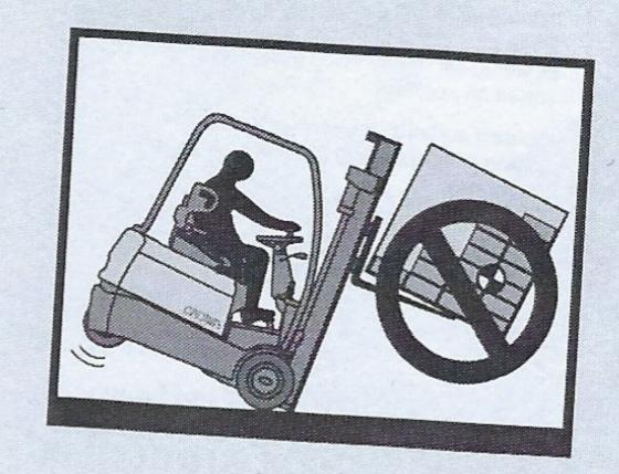
Check the carrying capacity of the floor before travelling on it. Do not exceed the maximum capacity for lifts and bridge decks. Make sure the bridge decks are secured.
