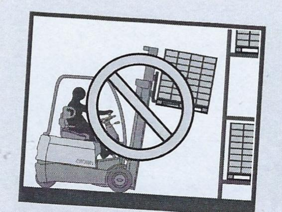
Keep the mast and the fork carriage vertical when storing or picking up a pallet.
