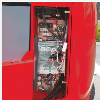
The controller is securely housed in the left side of the frame.
