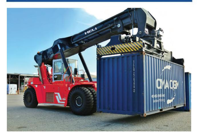
Anti slip stairways and safety handrails are fitted to the operator entry to the cabin accompanied by full length runningboards fitted to left and right hand sides of the Reach Stacker.
